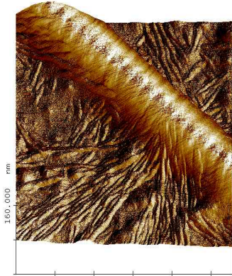
Atomic force microscopy of ex-vivo amyloid material
